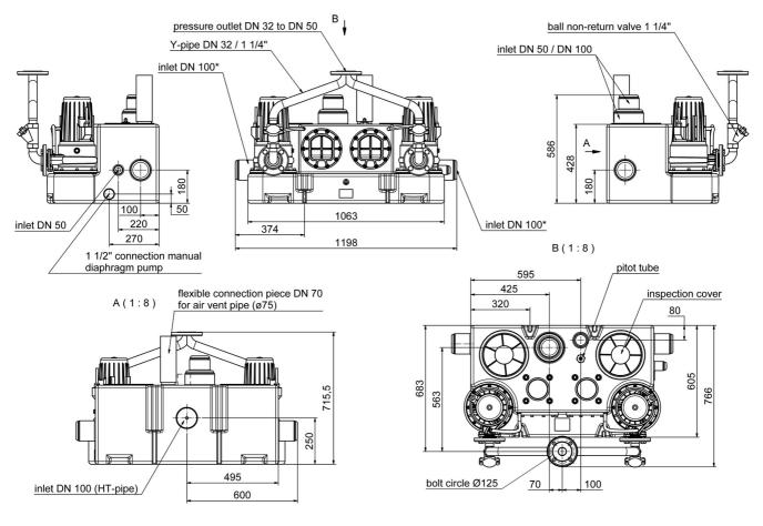
\*this inlet must be directed to a height of 250 mm above the ground level directly after the lifting unit
